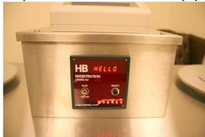
the photo-sensor at the counting station, to register counts on the light-to-dark transition (beam break) and display the current label count. The counter shows the number of times the light beam has been broken since the last counter reset. The counter also houses the Run/Setup Switch and the Counter Reset Button.
