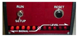
Next, move the web so that label is in the sensor's light beam. The lights to the **left** of center should be on when the label is positioned in the light beam, (light beam is broken by the label material plus backing).
