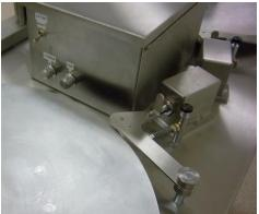
The tension control arm (two are installed on bidirectional label tables) is provided to ensure that as labels are being processed the tension of the label web remains constant. Tension is only applied to the "Supply" disk during label processing. This helps to ensure consistent label roll winding tensions and minimizes telescoping of labels as the labels are wound onto the take-up core.
