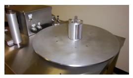
Your Scanning Devices Label Table has two 18" lift-off label discs with 3" mechanical core chucks. It is a bi-directional table which means you can count in both directions and both label disks are independently powered by two electronic motors installed on the underside of the label table. When counting in the forward direction, (left-to-right as you face the front of
