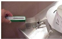
To determine the Tension setting, a "pull" tension gauge is applied to the flat riser on the Supply Reel Tension Control Arm. <u>Tension is only adjusted on the Supply Reel</u>, not the <u>Take-up Reel</u>. Once the correct tension is set, use the black locking dial to lock the adjustment screw in place.
