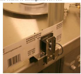
The sensor's vertical position is adjustable by loosening two set screws and moving the sensor up or down in the sensor bracket. Both sides (sensor and emitter must be adjusted to the same degree if the pair are to work properly together. The emitter/detector components should be positioned so that the label moves through the light beam and will be broken by the label at one point for each label. A small screwdriver is required to loosen the components for movement and retighten when positioned.
