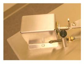
The electric brake is offered as an option on label tables with features that require fast stops of the label web for inspection of missing labels, mis-matched bar codes, or splices. The Electronic Brake will engage to stop the web when a missing label is detected. This feature will also automatically release pressure from the tension control arm and the take-up real when counting/processing begins.
