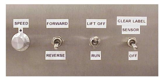
The panel hangs below the right side surface of the table and provides controls to power the table motors as well as to setting features of the table. The primary controls of a Scanning Devices Label Table are as follow from Left to Right in the picture above:
