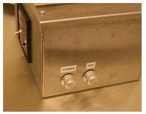
Adjust light sensitivity using the course and fine dials on the right side of the center console. Use the "coarse" dial first and the "fine" dial second. Adjust so that at least three lights are illuminated on the left side of the display panel when the label is positioned in the sensor's light beam. The more LEDs that light on each side during the adjustment process, the better the counting accuracy.
