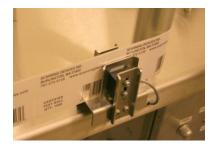
D. Pass the label web through the counting station web guide and counting station. Feed the label web in front of the right hand label guide and then wrap the label web leader around the take-up spindle, or tape the leader to the empty label core. Always wrap the labels around the take-up core in a counter-clockwise direction.
