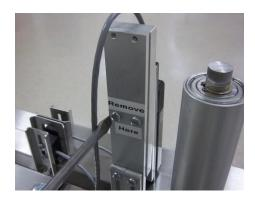
To remove the clear label sensor, simply remove the four screws on the back of the Clear Label Sensor Bracket also labeled "Remove Here". <u>DO NOT REMOVE THE CLEAR LABEL SENSOR BRACKET CONNECTED TO THE LABEL TABLE.</u> Once the four attachment screws are removed, the clear label sensor spacer and clear label sensor can be removed from the counting station area, or the sensor can be raised or lowered as needed.
