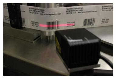
The Barcode Verification system is designed to read barcodes on labels as they move through the counting station to insure that barcodes are readable and correct. The counting sensor triggers the barcode scanner on the leading edge of the label. The barcode scanner attempts to read the label's code, compare it to the Target Barcode (the expected or "correct" code) and report the result.
