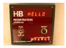
The counter's setup switch puts the counter in "Set-Up" mode allowing sensitivity adjustments for best optical contrast and sensing between label on web and spaces between labels. Adjusting the sensitivity to the specific label material being handled allows for the processing of a wide variety of label and label backing combinations.
