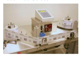
The labels to be processed are placed on the label disk on the left side of the label table (Supply Disk) with the labels unwinding from the left side, (counterclockwise rotation). The label web is fed in front of the left Label Web Guide with the backing facing the label guide. It then passes thru the counting station and across the front of the second label guide and is wrapped around a blank 3" corrugated core that is placed on the right side mechanical core
