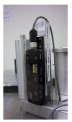
Your machine is provided with a clear label sensor shown here. This sensor is designed for counting clear labels on solid web backing or clear labels on clear web backing. The clear label sensor can be left in place when counting standard solid labels, it is recommended that the sensor is cleaned with some compressed air to remove any dust collection in the clear label sensor "sense" area.
