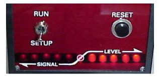
For best counting, the lights to the **right of center**, as shown in the photograph should be ON when the space between labels is positioned in the light beam (light projects through the label backing only). Adjust the sensitivity with the course and fine adjustment dials on the right side of the counter so that all five
