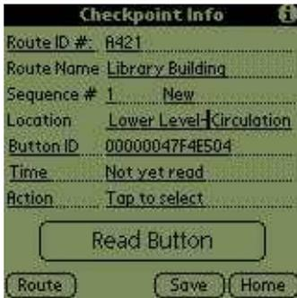
The iButton assigned to this checkpoint has been read and is displayed. This serial number will be stored in the Palm database with other checkpoint information. When the iButton is read on a route, it will be compared to this data to be sure that the individual is at the correct location.
