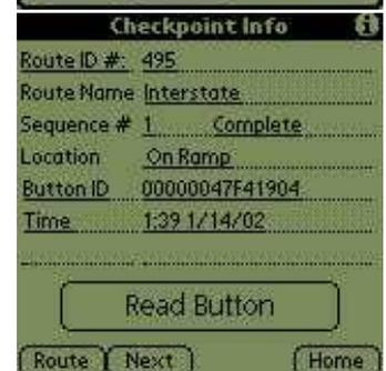
The next checkpoint on this route has a data entry requirement. First read the iButton to make sure you are at the right checkpoint. Again Palm Routes reads the iButton serial number and compares it to data stored in the Palm Database.
