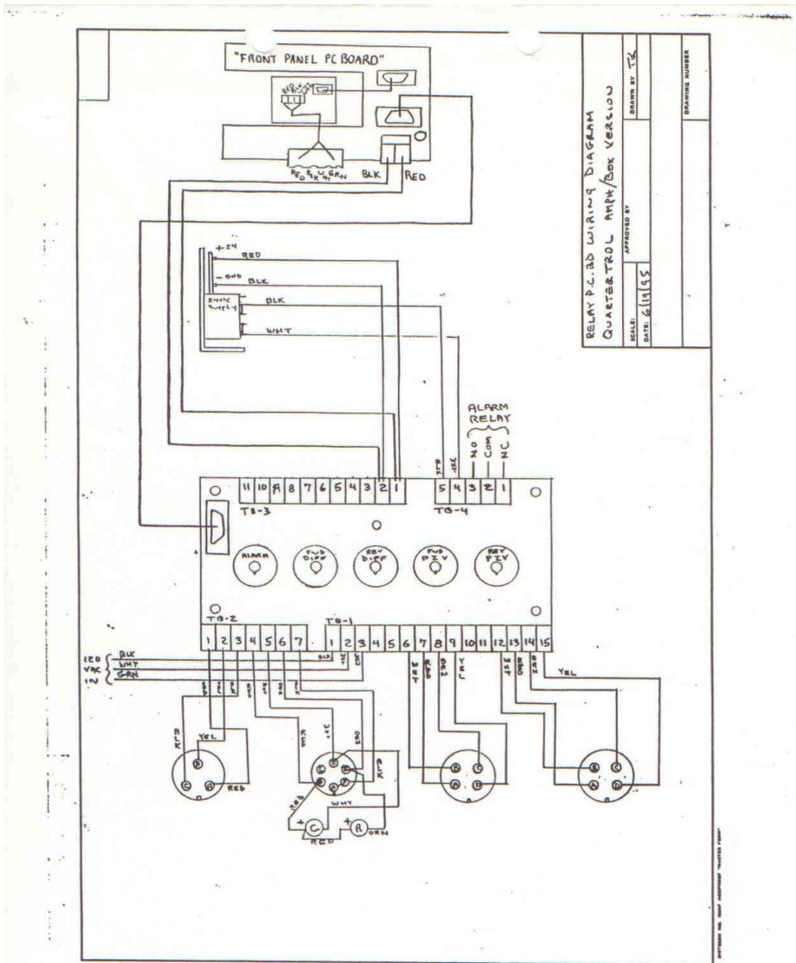
**Figure 2: Quarter-trol Output Module – Screw Terminal Connections**
