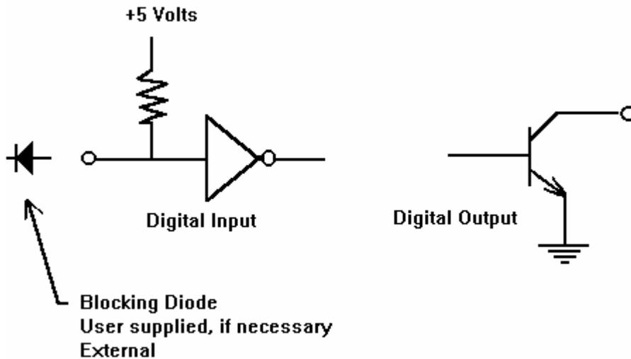
Digital inputs are logic gate inputs with a nominal 10 Kohm pull up resistor to +5 volts. These are designed for current sinking sensors or other current sinking devices. Sinking current (1/2 milliamp) from the input to signal ground asserts the input. **Do not apply external signals of more than 5 volts. Applying more than 5 volts to the digital input will cause immediate failure.** Use a blocking diode for connection to sensors which switch voltage instead of current.
