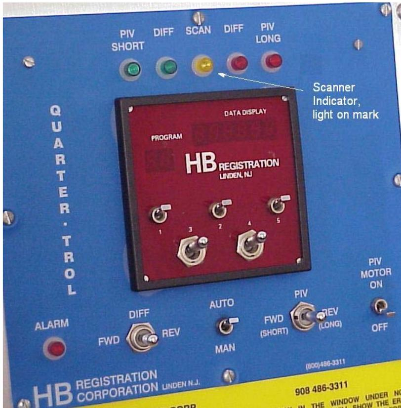
3. **Sympton:** Control is calling for correction larger than the window programmed.
