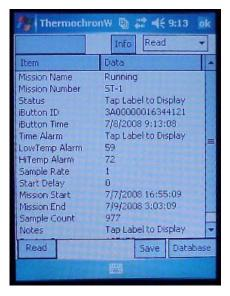
iConnection responds by reading the contents of the attached iButton and returning the data to the application. All thermochron mission parameters and data are read with a single tap on the Read button.
